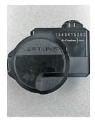
1. Locate meter and remove cap (if meter has one).
